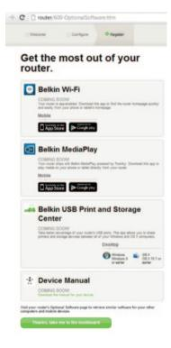
This screen shows you optional software that is available for your Modem Router, such as the USB software to allow you to print through the Modem Router's USB port. If you wish to download and install any of these software programs, simply click on the button appropriate for your device.
